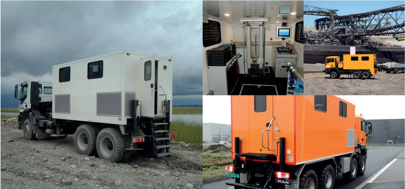
Geomil Equipment B.V. has come up with a new and universal concept for a fully ballasted all-terrain 200kN CPT sounding truck: the Grizzly-200.
